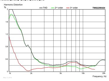
Measuring conditions, harmonic distortion Driver mounting: In "infinite" baffle Microphone distance: 0.5 m Input signal: Stepped sine wave, 2.83 VRMS Smoothing: 1/6 oct.
