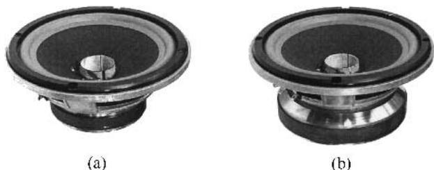
Fig. 25. Reference 8-in (203-mm) woofers used in experiments and modeling. (a) Loudspeaker A [long coil (12 mm), short gap (6 mm)]. (b) Loudspeaker B [short coil (6 mm), long gap (12 mm)].
